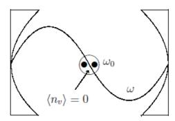
Figure. 1 The schematic of the model: a pair of two-level atoms possessing the transition frequency  $\omega_0$  embedded in a single-mode cavity with frequency  $\omega$ . In proposed model atomic pair is laser cooled and trapped in the ground vibrational state with vibronic quantum number  $\langle n_v \rangle = 0$ .
