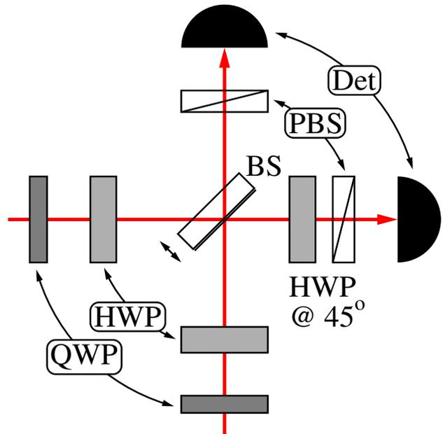
FIG. 1. Experimental setup for tomographical measurements. HWP – half-wave plate, QWP – quarter-wave plate, BS – non-polarizing beam splitter, PBS – polariser, Det – detector. For local measurements the BS is shifted out and the rotation of HWP behind is set to zero.
