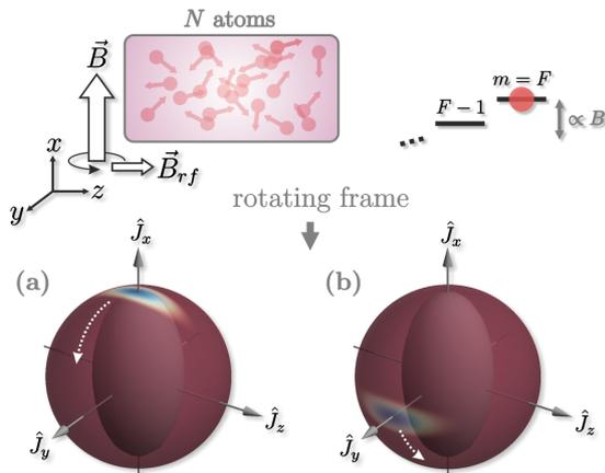
FIG. 1. Atomic magnetometry setup of [5], and the two potential preparation scenarios (a)/(b) of the atomic ensemble, yielding presented *squeezed* collective angular-momentum distributions.
