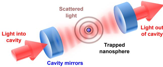
FIG. 1. Schematic of the experimental set-up for the quantum control of a levitated dielectric nanosphere within an optical cavity.
